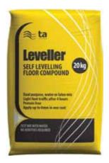
Leveller is a fast setting, cement based formulation for smoothing rough and uneven floors in preparation for laying a new floor covering. Leveller provides an ideal base for many floor coverings. Leveller is easily spread and can be applied up to depth of 6mm in one application, when mixed with 3mm – 5mm aggregate, Leveller can be applied up to a depth of 15mm. Used as instructed, Leveller will start to cure after 90 minutes and is ready to receive light foot traffic after 3 hours.
